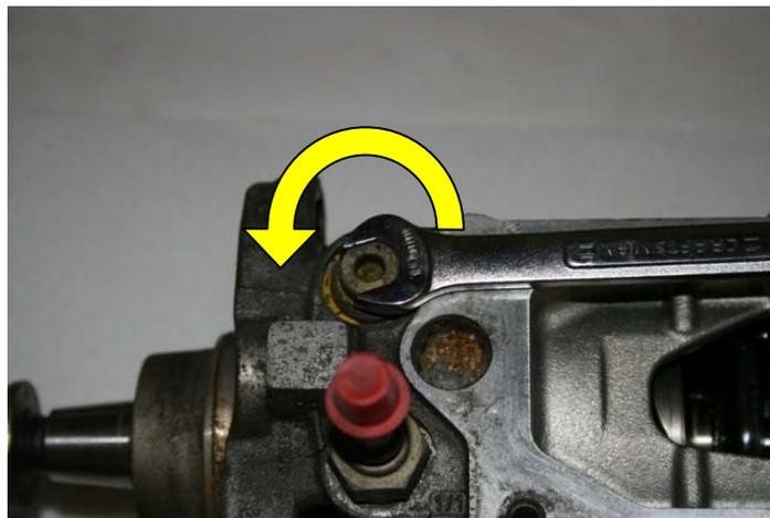
Loosen and remove the pressure regulating valve. There is a chance that the internal spring and plunger and expansion sleeve are down in the pump, use a magnet to extract the spring and steel plunger along with the expansion sleeve.
