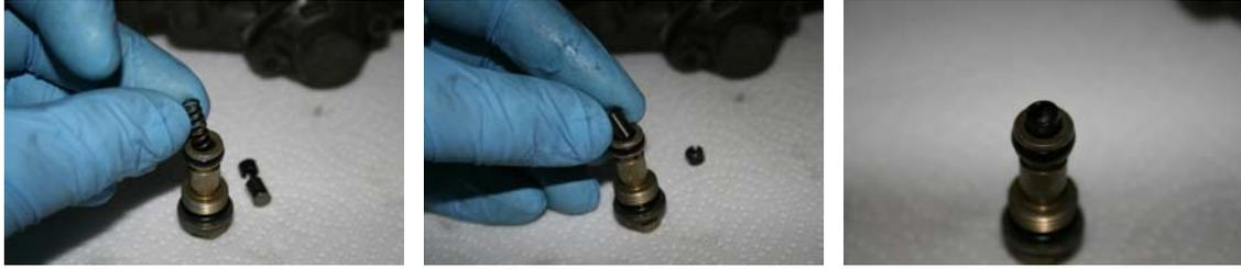
Use a pair of Channel locks to press the expansion spring back into the body of the pressure regulator until flush with the top.
