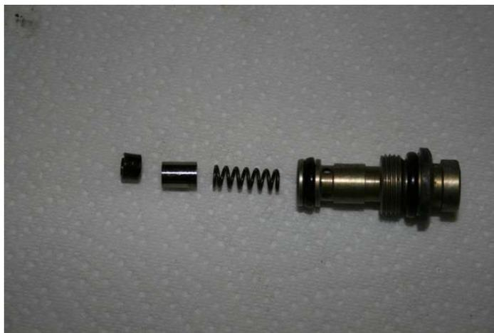
If the pressure regulator is intact, verify the internal steel plunger moves freely within the brass bore, this will tell you if the valve is able to compensate for pressure.
