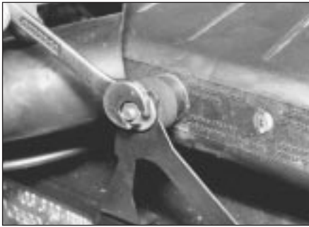
32.4b ... loosen front mounting nut ...
