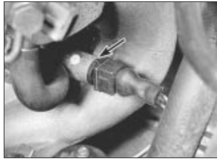
10.3 Auxiliary air valve (arrowed)
