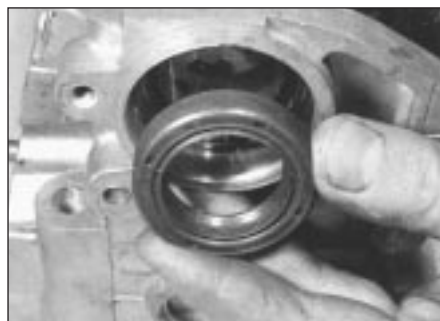
10.15 Removing camshaft oil seal
