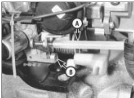
16.8 Idle speed adjustment screw and guide sleeve (A) mixture screw (B)
