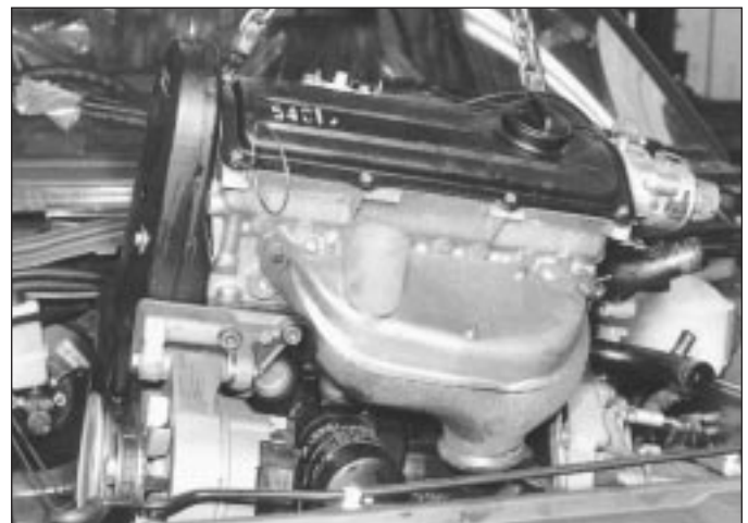
5.28 Lifting out engine/gearbox unit
