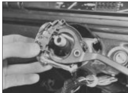
12.7a . . . and wiper control switch
