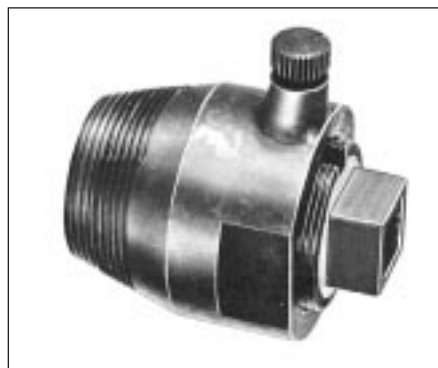
20.8 VW tool 2085 for removing crankshaft oil seal (timing belt end) and camshaft oil seal
