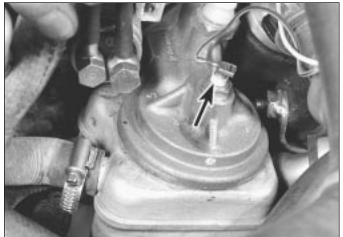
5.39 Oil temperature sender (arrowed)
