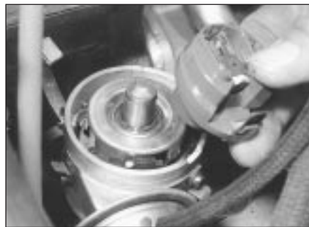
7.3a Pull free the rotor . . .
