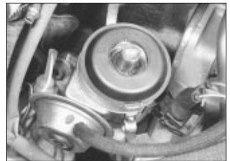
7.3b . . . and lift off the dust cap
