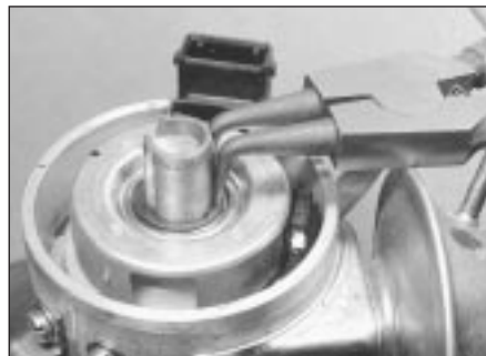
7.4a Remove the locking ring and rotor . . .
