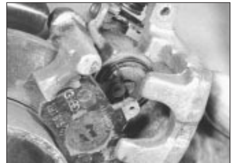
2.17 Rear brake caliper removal
